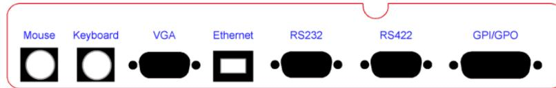
Figure 55: Satellite Console Rear Panel Connections
